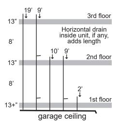
Some drains on the 3rd floor drain 19 ft straight down.
